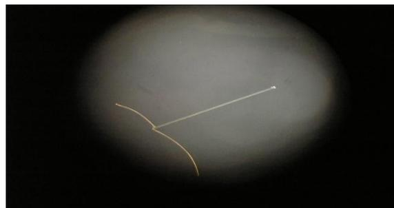
**Fig. 25.** Microthermocouple based on a bifilar MW.
