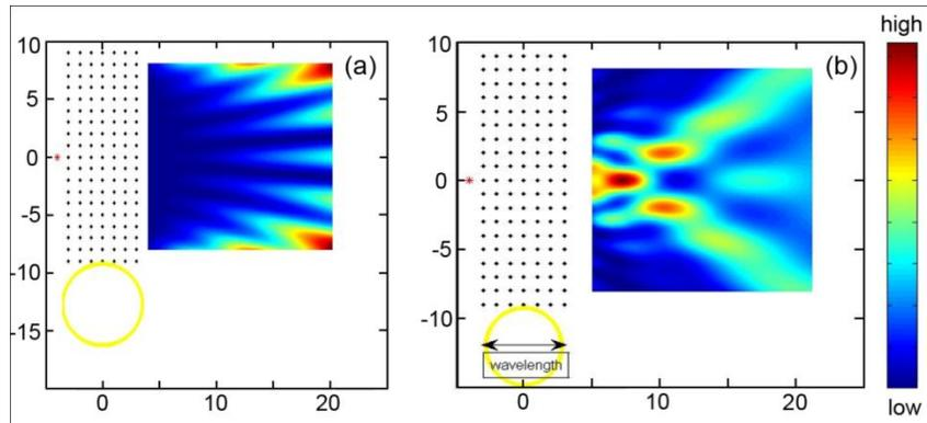
Fig. 5. Electric field intensity map of a cross-sectional view of the 2D source–image system when imaging by a photonic crystal slab consisting of a square lattice of cylinders calculated at inverse wavelength values of 0.58 (a) and 0.72 (b). The diameter of the circle in the figure corresponds to the wavelength.
