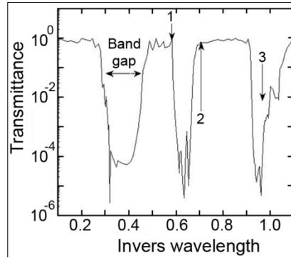
Fig. 3. Transmission coefficient for a photonic crystal composed of cylinders arranged in a square lattice.
