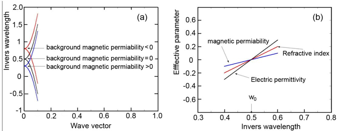
Fig. 1. (a) Dispersion curves at a singularity of a photonic crystal embedded in the “ether” with the background magnetic permeability. (b) Dependence of the effective parameters on the inverse wavelength.
