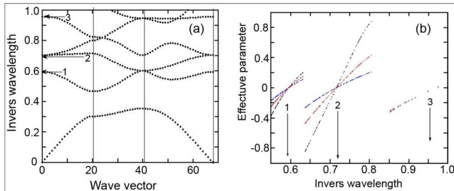
Fig. 2. (a) The band structure of a photonic crystal. (b) The effective parameters as a function of the inverse wavelength calculated for three singularity points.
