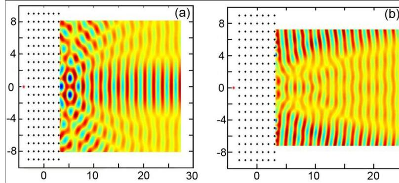
Fig. 4. Distribution of the electric field perpendicular to the plane  $E(x,y)$  calculated at inverse wavelength values of 0.58 (a) and 0.72 (b).
