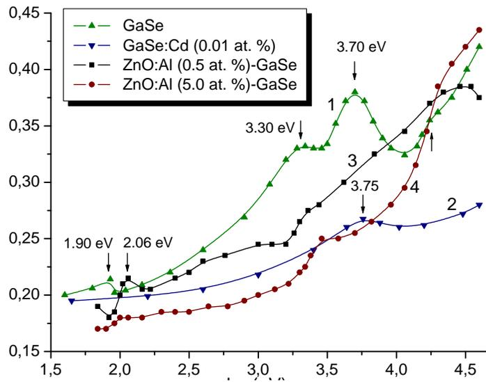
Fig. 3. Reflection spectra from the (0001) surface of the  $\epsilon$ -GaSe undoped lamella (1), the one doped with 0.01 at % Cd (2), and from the surface of ZnO:Al layer of ZnO:Al–GaSe heterojunctions for two aluminum concentrations: 0.5 at % (3) and 5.0 at % (4).
