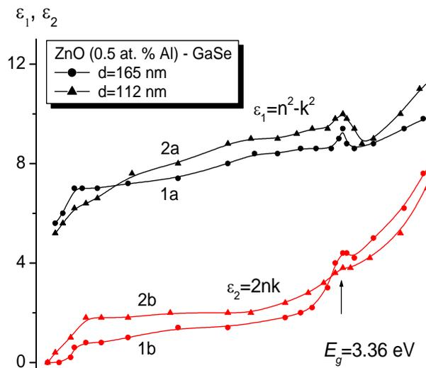
Fig. 4. Spectral distribution of the optical functions  $\epsilon_1(h\nu)$  and  $\epsilon_2(h\nu)$  for ZnO (0.5 at % Al) films having thicknesses of 165 (1) and 112 nm (2).
