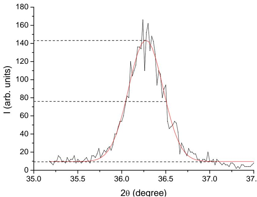
Fig. 2. Contour of the diffraction line corresponding to the  $2\theta=36.27^\circ$  for the (101) oriented ZnO:Al crystallites.
