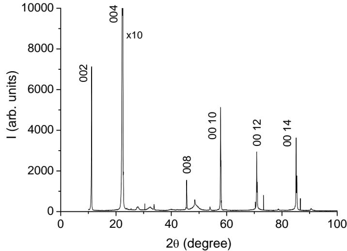
Fig. 1. XRD pattern of as-deposited sample of GaSe doped with Cd (0.01 at %).
