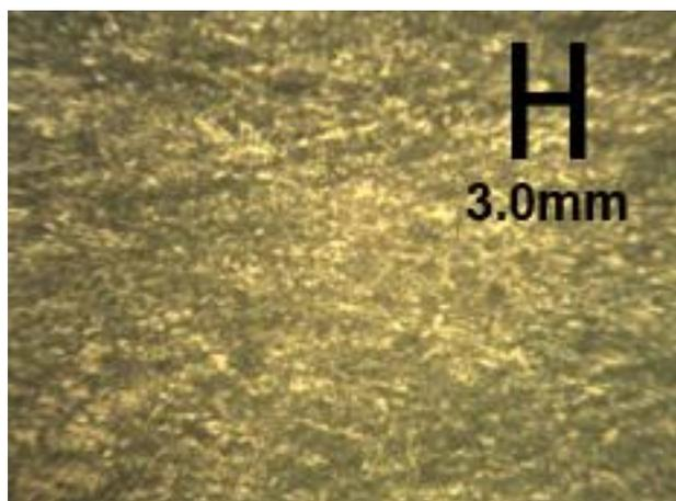
Fig. 6 a) Photo micrograph of ZnNiS ( $H_{11}$ )
