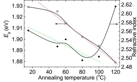
Fig. 4b. Dependence of the optical band gap  $E_g$  and refractive index  $n$  versus the annealing temperature  $T_{an}$  for amorphous  $\text{As}_{45}\text{S}_{15}\text{Se}_{40}$  thin films.
