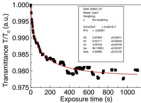
Fig. 5a. The kinetics of photodarkening during the light exposure for amorphous  $\text{Ge}_{0.07}\text{As}_{0.07}\text{Se}_{0.86}$  thin films.
