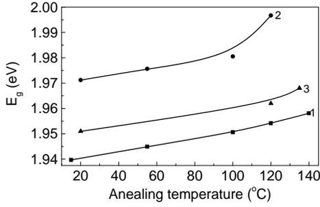
Fig. 4a. Dependence of the optical band gap  $E_g$  versus the annealing temperature  $T_{an}$  for amorphous (1)  $\text{Ge}_{0.09}\text{As}_{0.09}\text{Se}_{0.82}$ , (2)  $\text{Ge}_{0.18}\text{As}_{0.18}\text{Se}_{0.64}$ , and (3)  $\text{Ge}_{0.25}\text{As}_{0.25}\text{Se}_{0.50}$  thin films.
