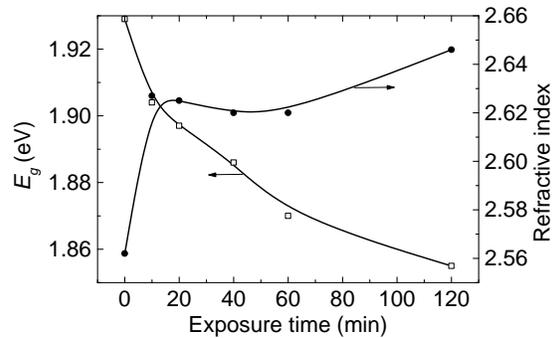
Fig. 2b. Dependence of the optical band gap  $E_g$  and refractive index  $n$  versus the exposure time  $t_{exp}$  for amorphous  $\text{As}_{45}\text{S}_{15}\text{Se}_{40}$  thin films.
