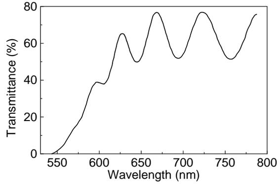
Fig. 1b. Transmission spectra of amorphous  $\text{As}_{45}\text{S}_{15}\text{Se}_{40}$  thin film ( $d=2.4 \mu\text{m}$ ).
