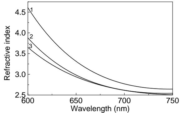
Fig. 3b. Dispersion curves of the refractive index  $n$  for amorphous  $\text{Ge}_{0.25}\text{As}_{0.25}\text{Se}_{0.50}$  thin films annealed at different temperatures  $T_{an}$ , °C: (1) 20, (2) 120, and (3) 135.
