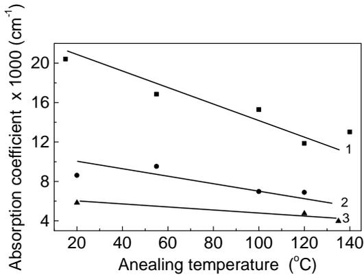
Fig. 3a. Dependence of the absorption coefficient  $\alpha$  versus annealing temperature  $T_{an}$  for amorphous (1)  $\text{Ge}_{0.09}\text{As}_{0.09}\text{Se}_{0.82}$ , (2)  $\text{Ge}_{0.18}\text{As}_{0.18}\text{Se}_{0.64}$ , and (3)  $\text{Ge}_{0.25}\text{As}_{0.25}\text{Se}_{0.50}$  thin films.
