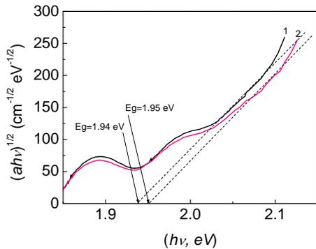
Fig. 2a. Dependence  $(\alpha hv)^{1/2}$  vs.  $(hv)$  for amorphous  $\text{Ge}_{0.05}\text{As}_{0.04}\text{Se}_{0.90}$  thin films: (1) as-deposited and (2) exposed for 2 h. The dashed line is a computing fitting giving the value of  $E_g$ .
