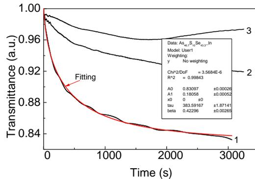
Fig. 5b. The kinetics of photodarkening in amorphous  $\text{As}_{45}\text{S}_{15}\text{Se}_{40}$  (curve 1),  $\text{As}_2\text{Se}_3$  (curve 2), and  $\text{As}_2\text{S}_3$  (curve 3) thin films.
