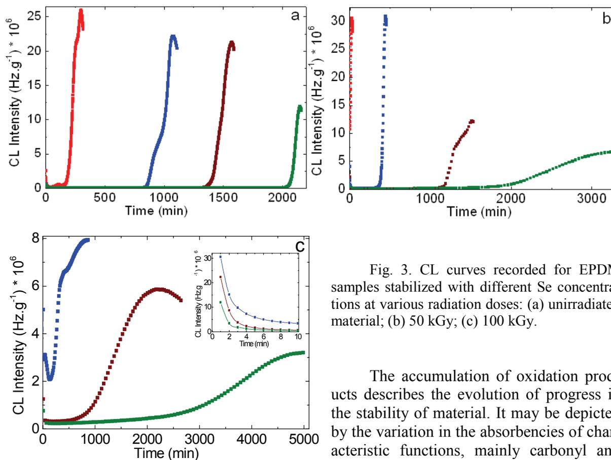
Fig. 3. CL curves recorded for EPDM samples stabilized with different Se concentrations at various radiation doses: (a) unirradiated material; (b) 50 kGy; (c) 100 kGy.
