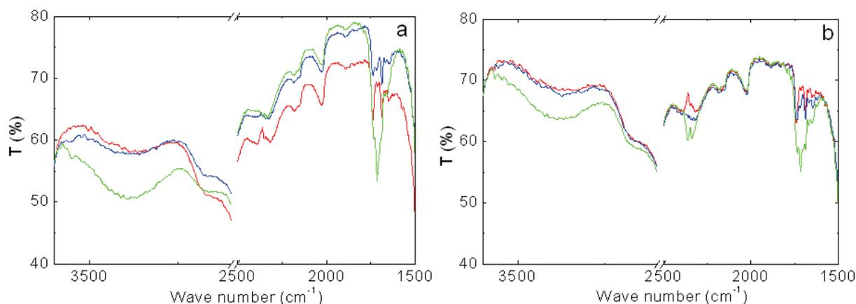
Fig. 4. FTIR spectra recorded for EPDM samples stabilized with different Se concentrations: (a) pure sample and (b) 0.5% metallic Se.
