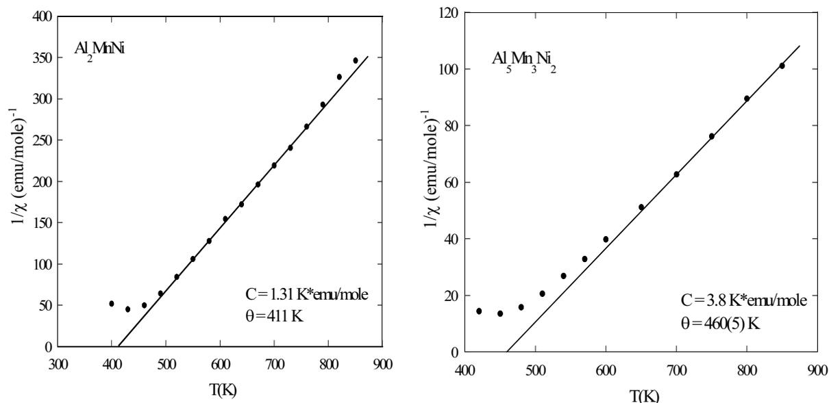
Fig. 3. Thermal variation of the reciprocal susceptibility of  $\text{Al}_2\text{MnNi}$  and  $\text{Al}_5\text{Mn}_3\text{Ni}_2$
