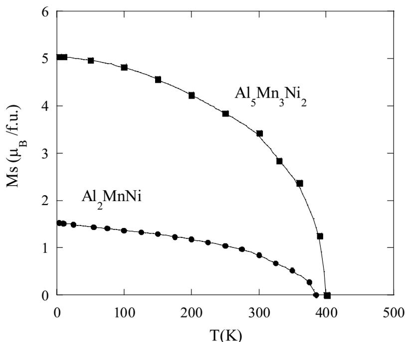
Fig. 2. Thermal variation of the spontaneous magnetization of  $\text{Al}_2\text{MnNi}$  and  $\text{Al}_5\text{Mn}_3\text{Ni}_2$ .
