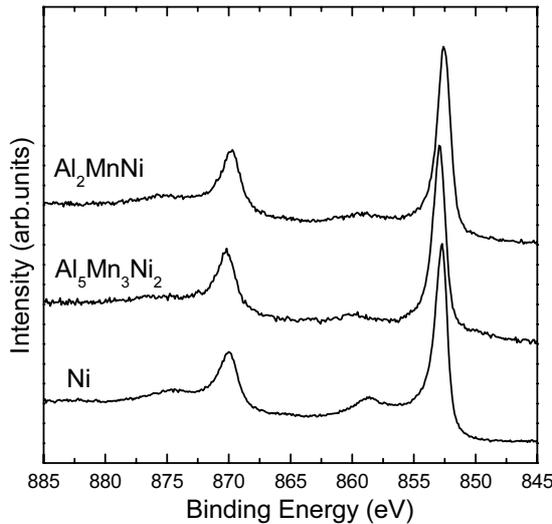
Fig. 5. XPS Ni 2p core level spectra of Al<sub>2</sub>MnNi, Al<sub>5</sub>Mn<sub>3</sub>Ni<sub>2</sub> and metallic Ni.
