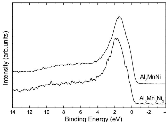
Fig. 6: XPS valence-band spectra of  $\text{Al}_2\text{MnNi}$ ,  $\text{Al}_5\text{Mn}_3\text{Ni}_2$
