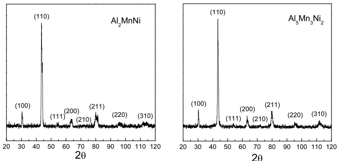
Fig. 1. X-ray diffraction pattern of  $\text{Al}_2\text{MnNi}$  and  $\text{Al}_5\text{Mn}_3\text{Ni}_2$ .
