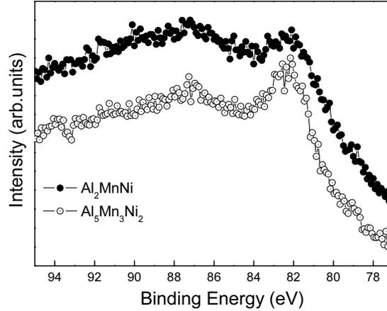
Fig. 4. XPS Mn 3s core level spectra of Al<sub>2</sub>MnNi and Al<sub>5</sub>Mn<sub>3</sub>Ni<sub>2</sub>.
