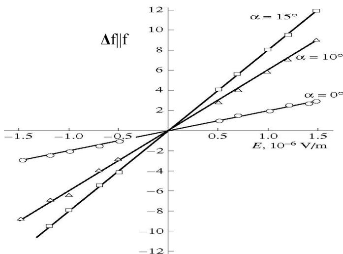
Fig. 5. Linear dependence of the relative change in the frequency on the constant electric field for three orientations of the langasite rods vibrating in the compression-tension mode along the length.
