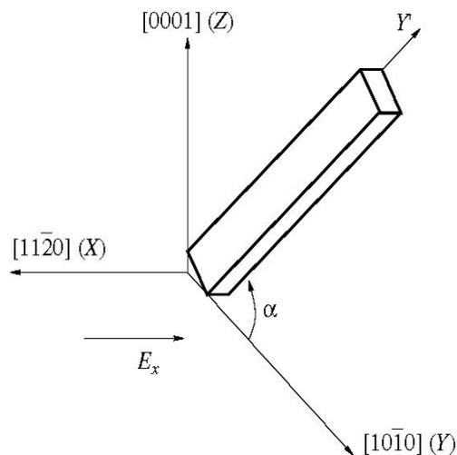
Fig. 4. Shape and crystallographic orientation of the langasite crystals.
