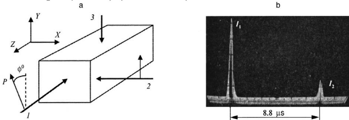
Fig. 2. (a)-Interaction geometry of transverse sound wave (1) with polarization  $P$ , light wave (2) polarized along  $X$ , and electric field  $E(3)$  in a LiTaO<sub>3</sub> crystal; (b)-diffraction pulses ( $I_1$ ) and ( $I_2$ ), induced by the incoming and reflected sound pulses, respectively.
