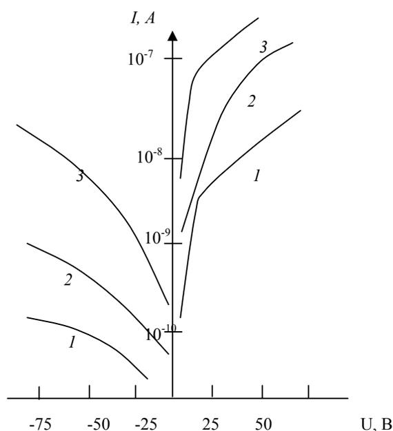
Fig.1. Dark I-V characteristic of the heterostructures GaAs-As<sub>2</sub>Se<sub>3</sub> at different temperatures T°C: 1 – 20; 2 – 50; 3 – 75
