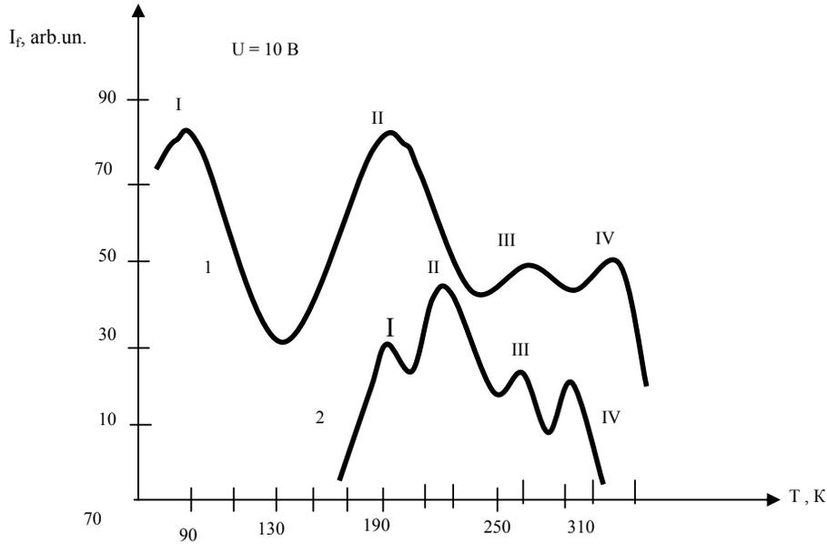
Fig.5. Thermostimulated currents of the GaAs-As<sub>2</sub>Se<sub>3</sub> heterostructures: 1- back bias; 2- direct bias.
