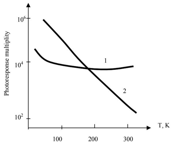
Fig.4. Dependence of the photoresponce multiplicity of the GaAs-As<sub>2</sub>Se<sub>3</sub> heterostructures on temperature for U =10V at the direct (1) and back (2) bias.
