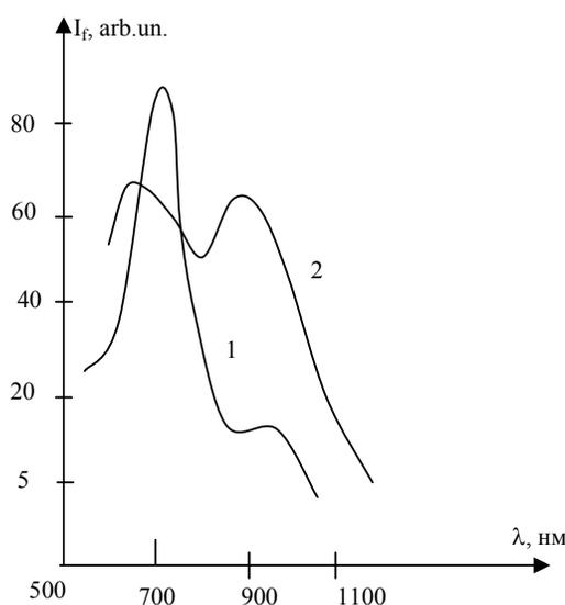
Fig.2 Spectral distribution of the photosensitivity of the GaAs-As<sub>2</sub>Se<sub>3</sub> heterostructures at T=300 K and at the direct (1) and back (2) bias of applied voltage
