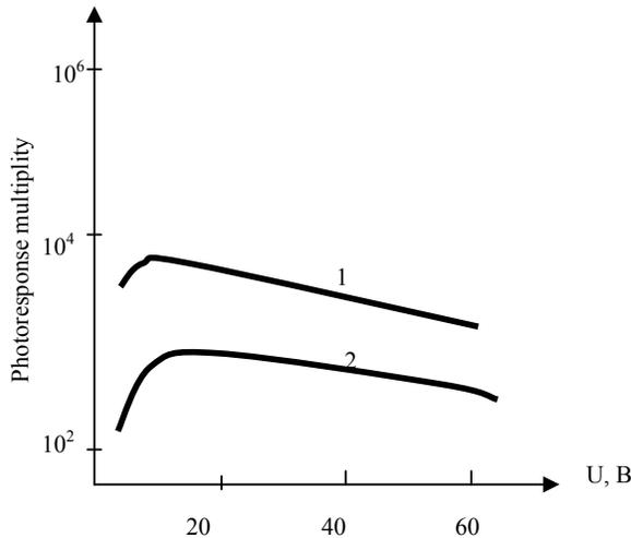
Fig.3. Dependence of the photoresponce multiplicity of the GaAs-As<sub>2</sub>Se<sub>3</sub> heterostructures at T=300K on applied direct (1) and back (2) bias.
