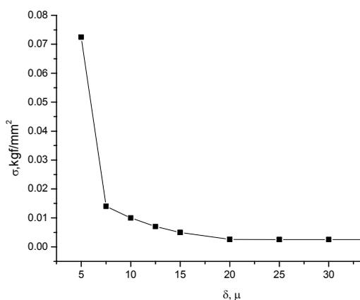
Fig. 4. The dependence of the wire tension on diameter.
