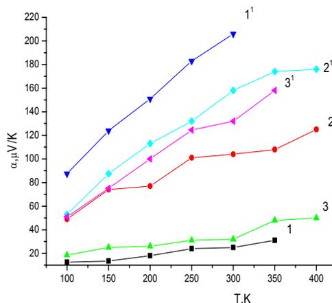
Fig.18. The temperature dependence of the thermopower of the samples of type n for nontreated wires (1, 2 and 3) and treated ones (1', 2' and 3').
