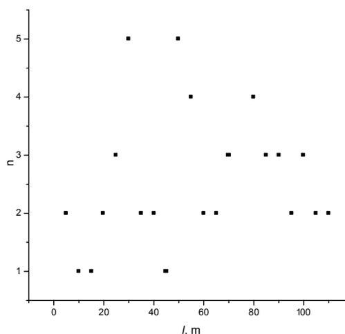
Fig. 3. Number of cracks of the core per 1 m of the microwire in the limits of one bobbin.
