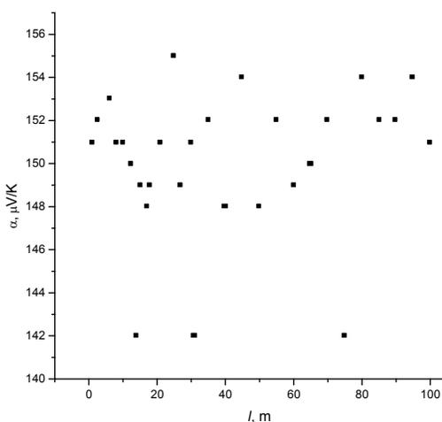
Fig.11. Dispersion of the Seebeck coefficient of the nontreated samples in the limits of one bobbin
