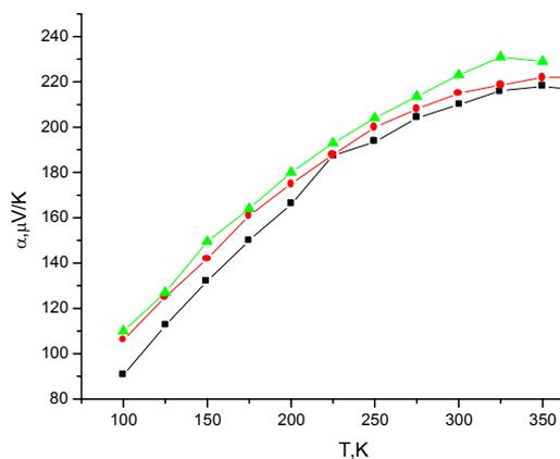
Fig.15. The temperature dependence of the thermopower of the samples of type p treated at the temperature 450 K in the time interval: 1 - 48 hours, 2 - 96 hours, 3 - 72 hours.
