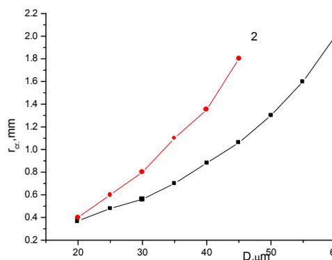
Fig. 8. The dependence of the critical radius of flexion on the cover diameter for nontreated samples (1) and the ones treated by annealing (2).
