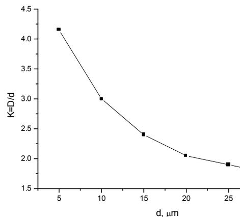
Fig. 6. The dependence of the ratio  $D/d$  on the microwire core diameter.
