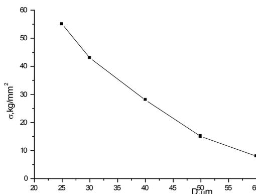
Fig. 7. The dependence of the microwire durability on the cover diameter for nontreated samples (1) and the ones treated by annealing (2).
