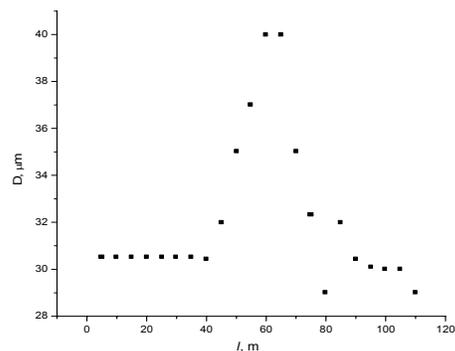
Fig. 2. Dispersion of the isolation diameter  $D$  lengthwise microwire in the limits of one bobbin.
