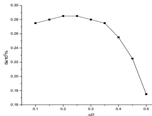
Fig.10. Change of tensosensitivity of the microwire core at its relative deformation.
