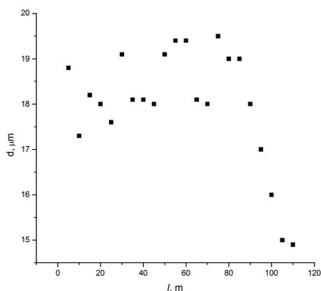
Fig. 1. Dispersion of the core diameter  $d$  lengthwise microwire in the limits of one bobbin
