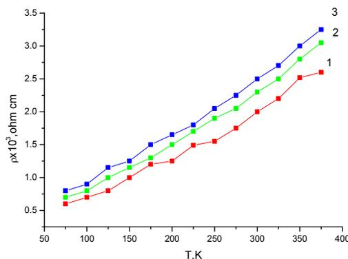
Fig. 16. The temperature dependence of the resistivity of the samples of type p treated at the temperature 450 K in the time interval: 1 - 1 hour, 2 - 72 hours, 3 - 96 hours.
