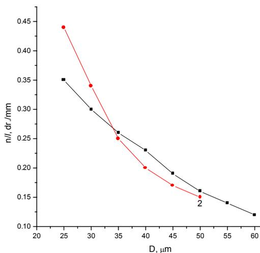
Fig.9. The dependence of number of limit of torsion per a unit of length of the microwire on the cover diameter for nontreated samples (1) and the ones treated by annealing (2).
