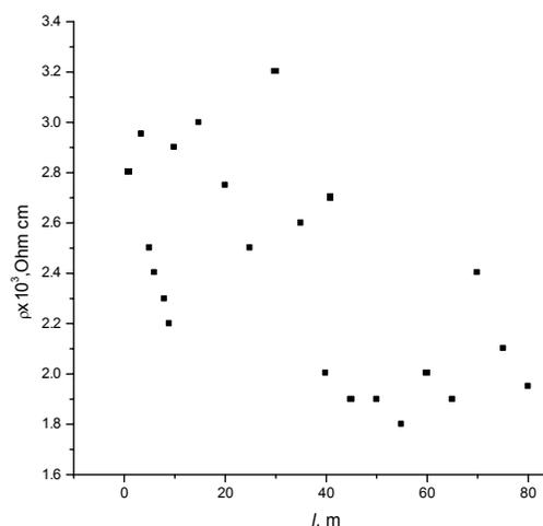
Fig.12. Dispersion of the resistivity of the nontreated samples in the limits of one bobbin.
