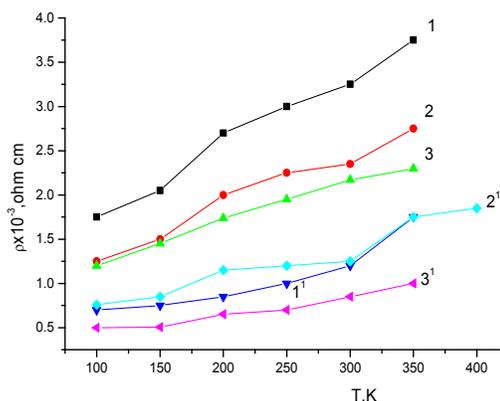
Fig. 17. The temperature dependence of the resistivity of the samples of type n for nontreated wires (1, 2 and 3) and treated ones (1', 2' and 3').
