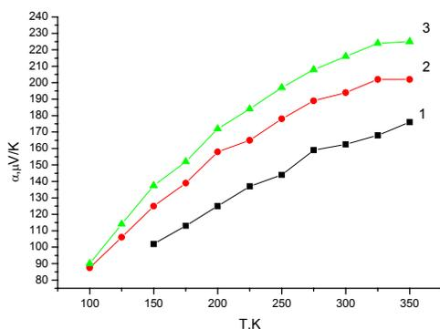
Fig.13. The temperature dependence of the thermopower of the samples of type p: 1 – before annealing, 2 - after annealing at the temperature 473 K, 3 - after annealing at the temperature 520 K. Time of annealing is 24
