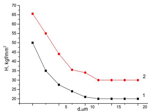
Fig. 5. The dependence of the microhardness on the microwire diameter.
